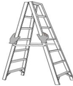
Figure 2-5 Personnel Ladder Support Diagram
