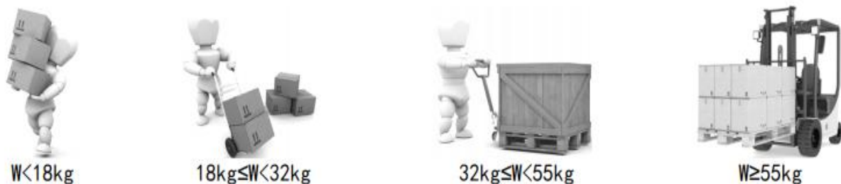
Figure 2-3: Schematic of Lifting Methods for Different Weight Loads
